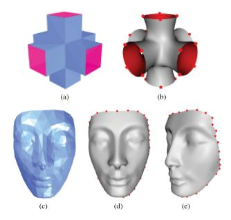
Fig.3. Open mesh examples (I-surface ≡ interpolating Loop surface). Red solid dots are boundary vertices of the given mesh.(a) (c) Given mesh. (b) (d) I-surface. (e) Different view.
