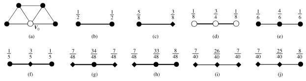
Fig.1. (a) Regular vertex. (b) $\sim$ (d) Boundary subdivision rules. (e) $\sim$ (j) Limit point forumlas. The solid circular points are regular vertices and rectangle points are extraordinary vertices.
