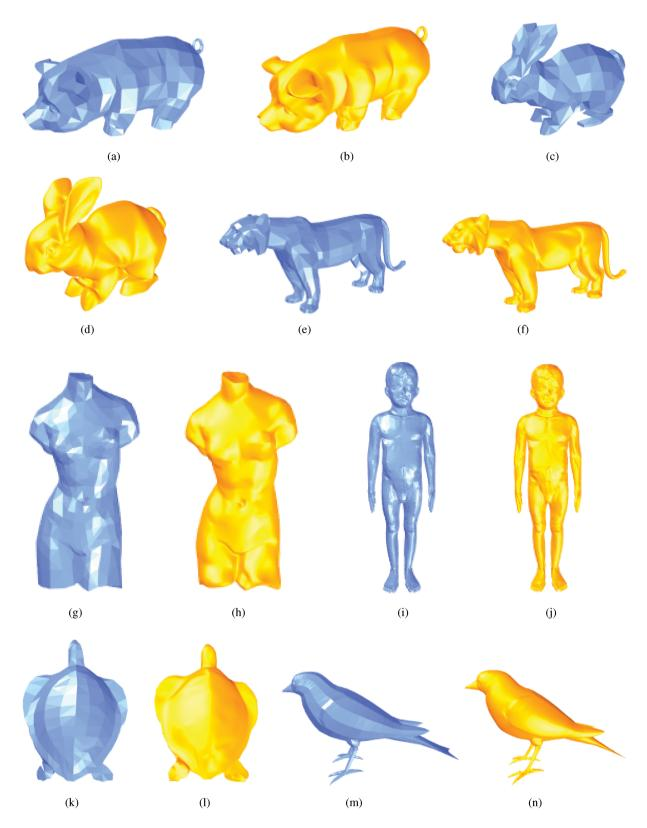
Fig.2. Examples of progressive interpolation using Loop subdivision surfaces (G-mesh  $\equiv$  given mesh; I-surface  $\equiv$  interpolating Loop surface). (a) (c) (e) (g) (i) (k) (m) G-mesh. (b) (d) (f) (h) (j) (l) (n) I-surface.
