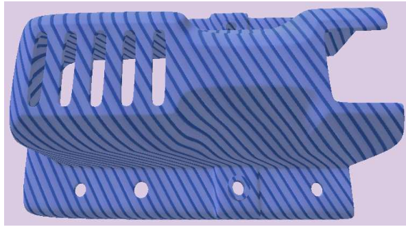
(b) Ventilation control component
