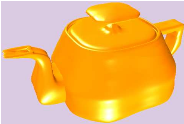
(c) Interpolating surface generated with user selected blending areas around upper portion of the teapot body
