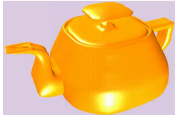
(d) Interpolating surface generated with user selected blending areas around bottom portion of the teapot body
